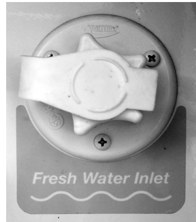
Fresh (City) Water Connection “Fresh Water Inlet” (Located on the driver's side sidewall) -Typical View
