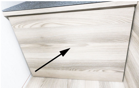
Winterization Valve #1 Pull off the cover to access- located in driver's side rear closet. -Typical View
