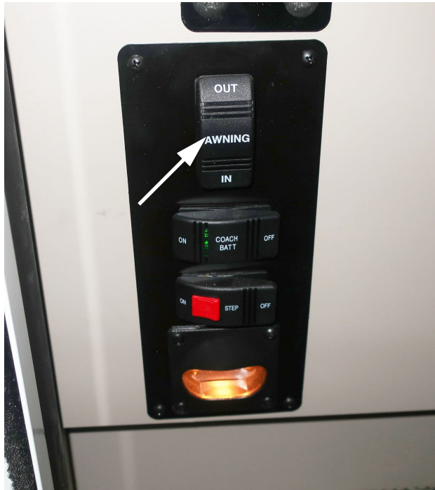
Power Awning control switch (Located near the entrance door) -Typical View
